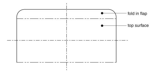
**(b)** The fold in flap needs to lock in place without the use of glue. In the space below use sketches and notes to show a design for a locking flap.
