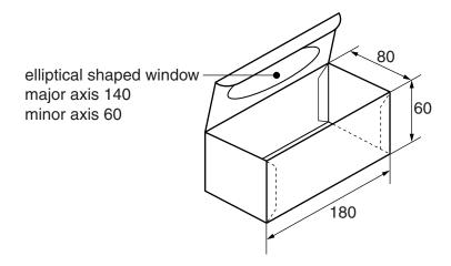
(a) Complete the scale 1:2 development (net) of the package for the biscuits below by:
