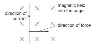
In which direction is the force when the current direction is reversed?
