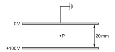
What is the electric field strength at point P midway between the plates?
