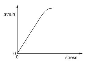
Why is the strain energy per unit volume of the material **not** the area under the graph?
