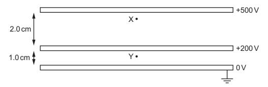
What is the value of the ratio  $\frac{\text{magnitude of force on an electron at X}}{\text{magnitude of force on an electron at Y}}$ ?
