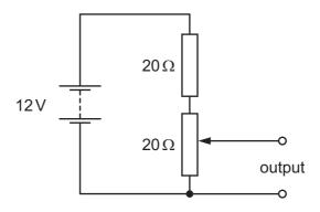
The fixed resistor and the potentiometer each have resistance  $20\Omega$ . The circuit is designed to provide a variable output voltage.
