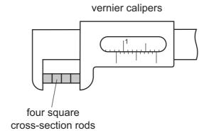
The measurement is  $(8.4 \pm 0.1)$  mm and the zero reading on the calipers is  $(0.0 \pm 0.1)$  mm.
