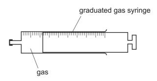
The volume of gas at room temperature is 2.0 cm<sup>3</sup>.
